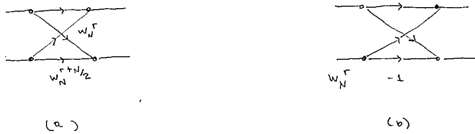
Fig. 3 (a) The butterfly which is the basic computational element of the FFT algorithm
