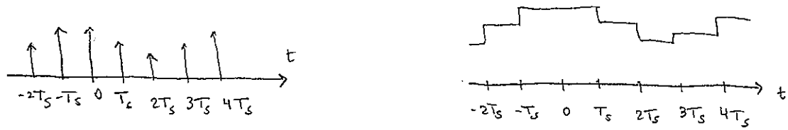
Fig. 6 The use of a zero-order hold to interpolate between the samples in x_s(t) .
