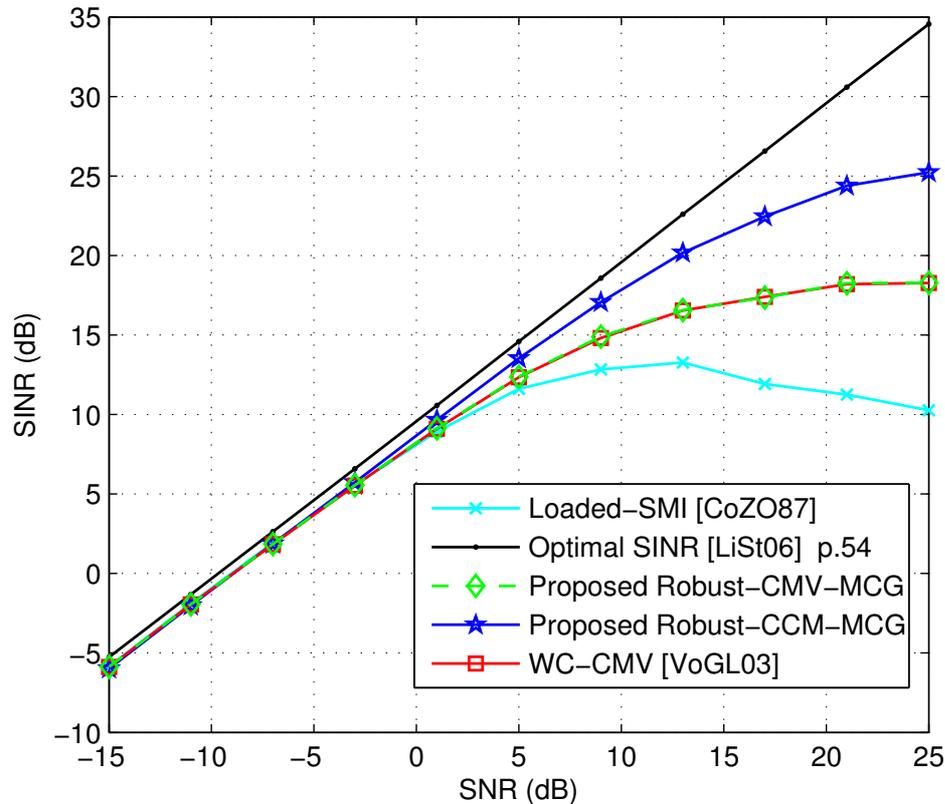
Figure 2.7: SINR performance versus SNR,  $i = 1500$
