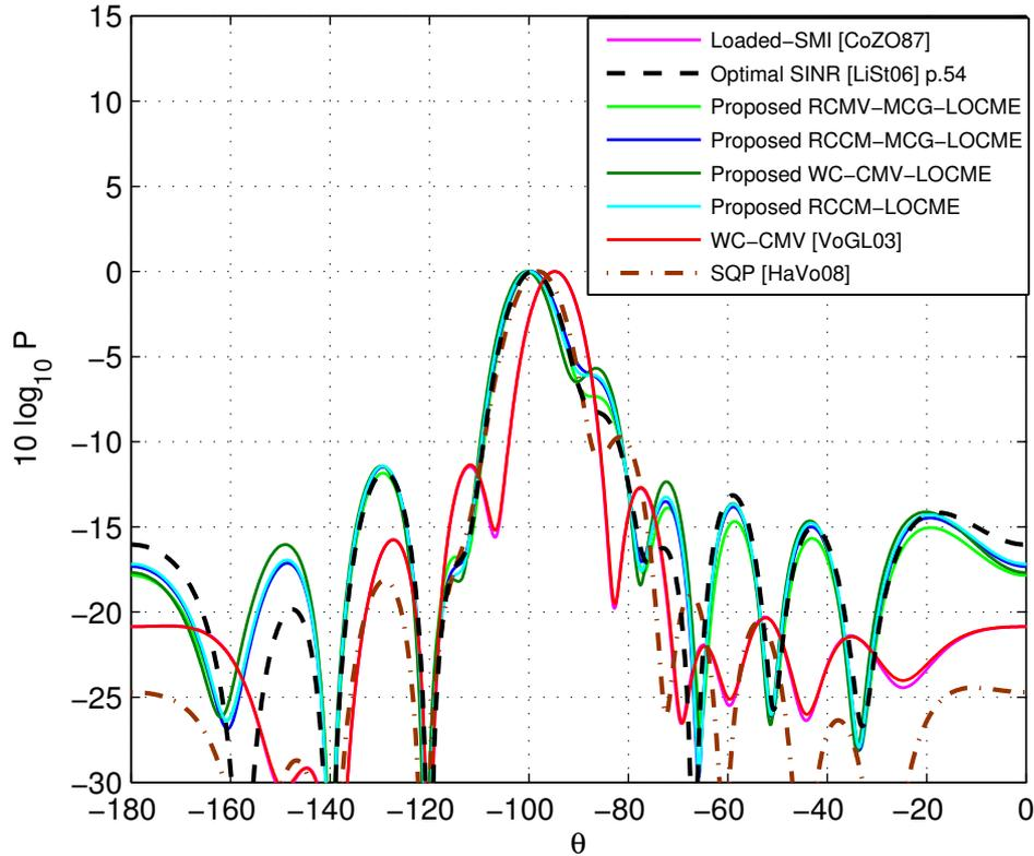
Figure 3.1: Beampattern, mismatch due to LCS, SNR = 0 dB,  $K = 2$ ,  $D = 5$
