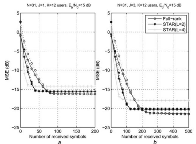
**Fig. 4** MSE for analytical and simulated results against the number of received symbols for processors with linear receivers using
