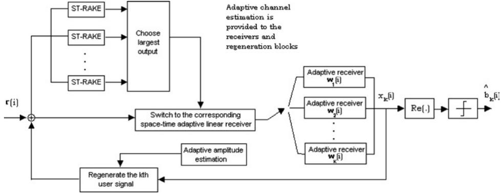
**Fig. 2** Proposed space-time adaptive SIC receiver
