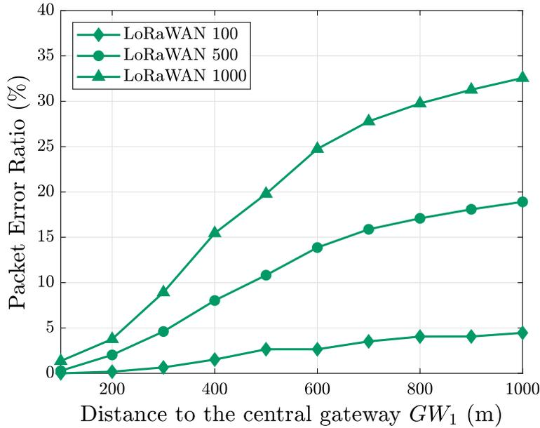
Figure 3.6: Average PER versus distance to the central gateway  $GW_1$  (Scenario 1). At the figure’s legend, “LoRaWAN  $N$ ” indicates that this curve corresponds to a LoRaWAN network with  $N$  nodes.
