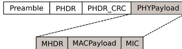
Figure 4.2: The message format of an RL-LoRa beacon, where PHDR is the LoRa physical header (PHDR), PHDR\_CRC is the latter’s Cyclic Redundancy Check (CRC), and PHYPayload is the physical payload. Inside the PHYPayload field, MHDR represents the MAC header, MACPayload is the MAC payload (it carries the RL-LoRa beacon fields), and MIC is a 4-bytes Message Integrity Code (MIC) [4].
