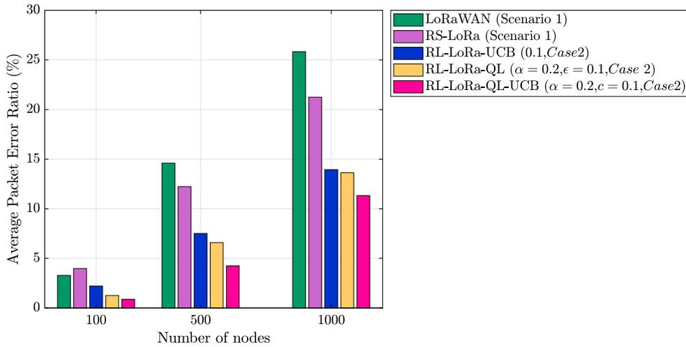
Figure 4.12: Average PER under LoRaWAN, RS-LoRa, RL-LoRa.
