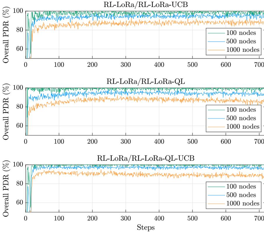
Figure 4.17: Average PDR versus steps of the RL algorithm under the proposed RL-LoRa/*RL-LoRa-UCB*, RL-LoRa/*RL-LoRa-QL*, and RL-LoRa/*RL-LoRa-QL-UCB* MAC protocols.
