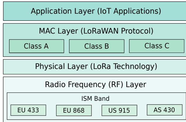
Figure 2.1: The network stack of LoRaWAN [1].
