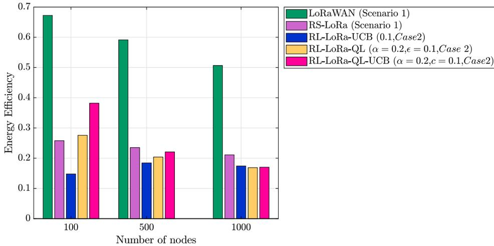
Figure 4.15: Energy efficiency under LoRaWAN, RS-LoRa, RL-LoRa.
