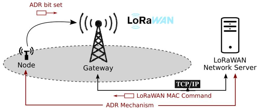
Figure 3.3: Adaptive Data Rate mechanism of LoRaWAN.
