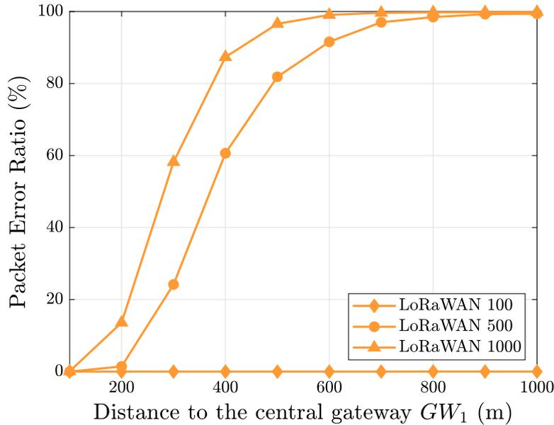
Figure 3.8: Average PER versus distance to the central gateway  $GW_1$  (Scenario 3). At the figure’s legend, “LoRaWAN  $N$ ” indicates that this curve corresponds to a LoRaWAN network with  $N$  nodes.
