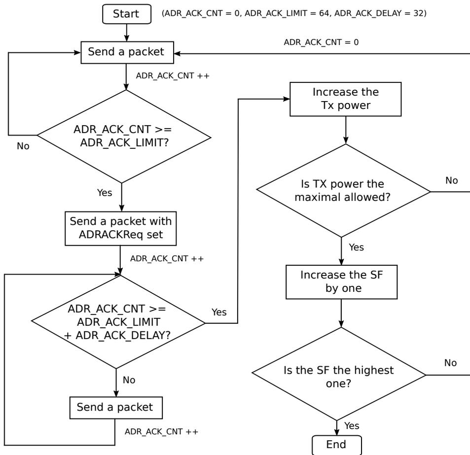
Figure 3.4: LoRaWAN ADR mechanism at the node's side, where “Tx power” represents the transmit power.
