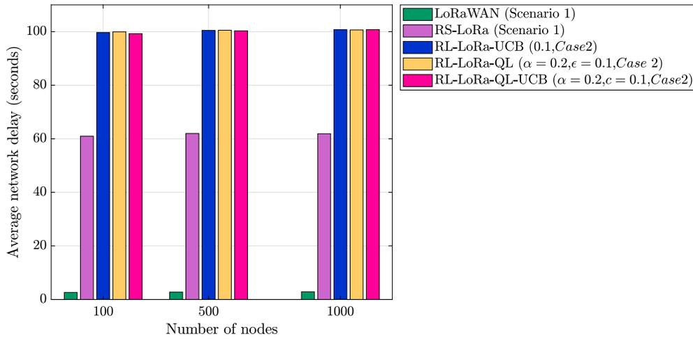
Figure 4.14: Average network delay under LoRaWAN, RS-LoRa, RL-LoRa.
