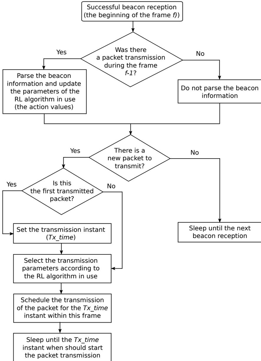
Figure 4.4: Procedure executed by nodes after a successful beacon reception.
