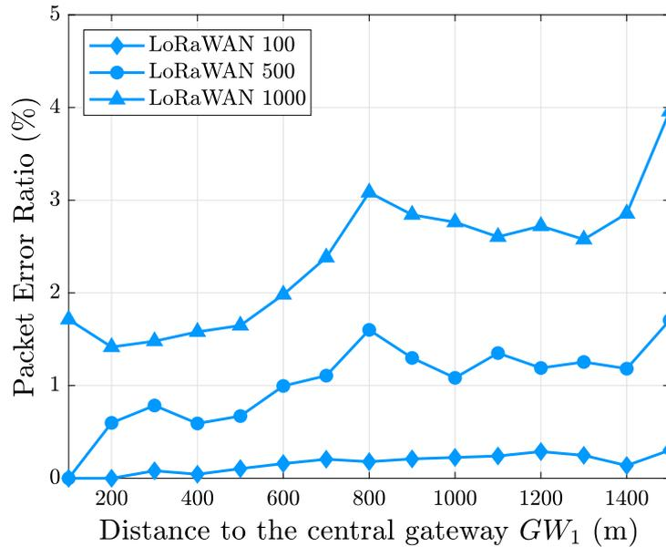
Figure 3.7: Average PER versus distance to the central gateway  $GW_1$  (Scenario 2). At the figure’s legend, “LoRaWAN  $N$ ” indicates that this curve corresponds to a LoRaWAN network with  $N$  nodes.
