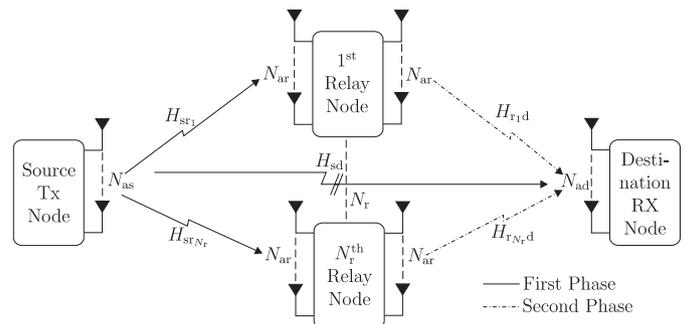
Fig. 1. MIMO multi-relay system model.
