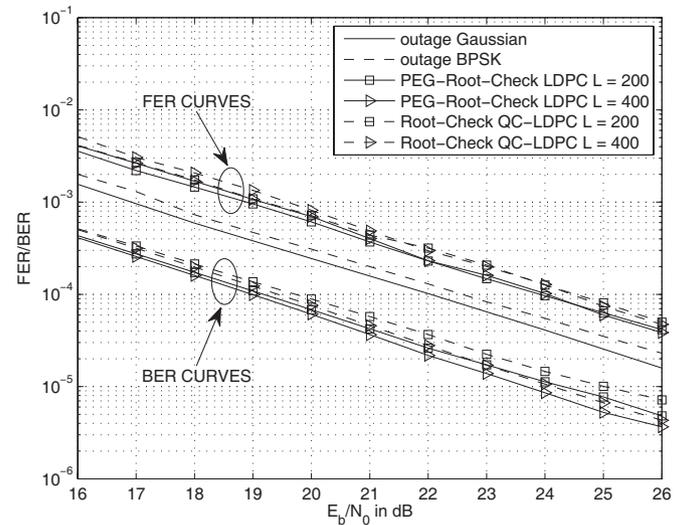
Fig. 2. FER and BER performance comparison for PEG-Root-Check LDPC codes and Root-Check QC-LDPC codes with codeword length  $L = 200$  and 400 bits over a block-fading channel with  $F = 2$ . The maximum number of iterations is 20.
