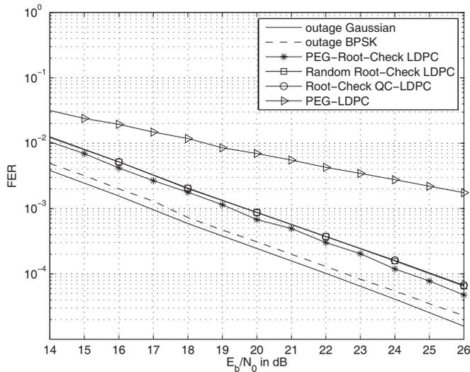
Fig. 1. FER performance comparison for Root-Check QC-LDPC codes, Random Root-Check LDPC codes, PEG LDPC codes and PEG-Root-Check LDPC codes over a block-fading channel with  $F = 2$  and  $L = 1200$ . The maximum number of iterations is 20.
