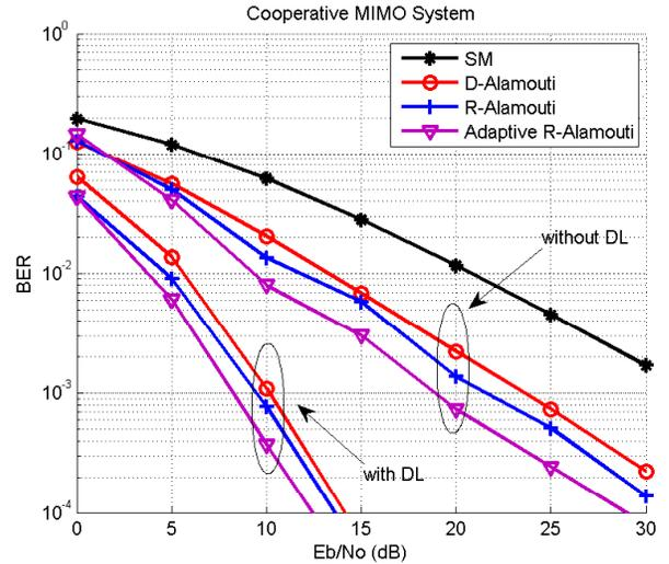
Fig. 3. BER performance v.s.  $E_b/N_0$  for ARMO Algorithm with and without the Direct Link
